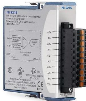
The NI-9215 performs differential analog input. The module contains NIST-traceable calibration, a channel-to-earth ground double isolation barrier for safety and noise immunity, and high-common-mode voltage range. It is also offered in two connectivity variants: 10-position screw terminal or BNC.
