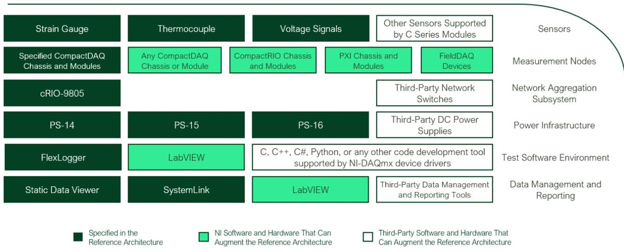
Figure 2. NI software and hardware tools are interoperable and are supported by, and support, a wide range of industry standard tools. The Static Structural Test Reference Architecture is a guide for designing a test system that has been validated and tested with performance metrics. If your specific requirements call for other tools, there is a good chance the components of the reference architecture can support you.
